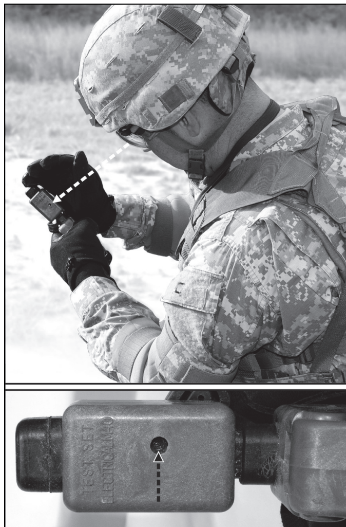
Figure 3-11. Conducting a circuit test of the M57 firing device while observing the window on the M40 test set
