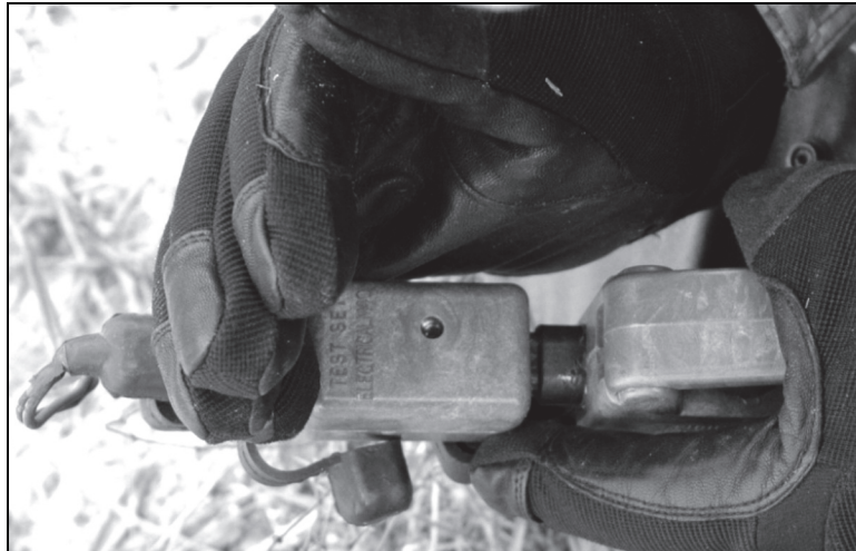
Figure 3-17. Conducting a circuit test of the firing wire while observing the window on the M40 test set
