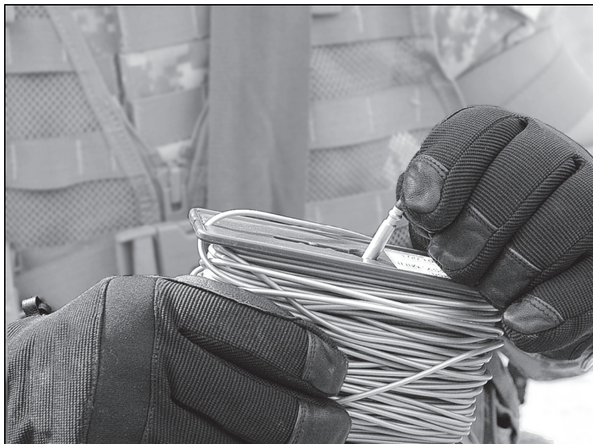
Figure 2-9. Removing the nonelectrical blasting cap from the spool at the munition emplacement site
