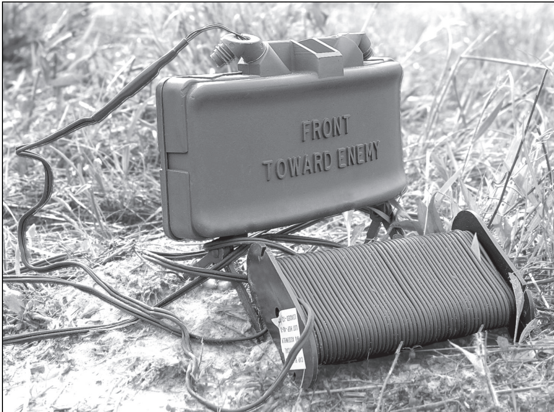
Figure 3-25. Placing the firing wire spool with remainder of spooled wire in front of the M18A1 claymore munition
