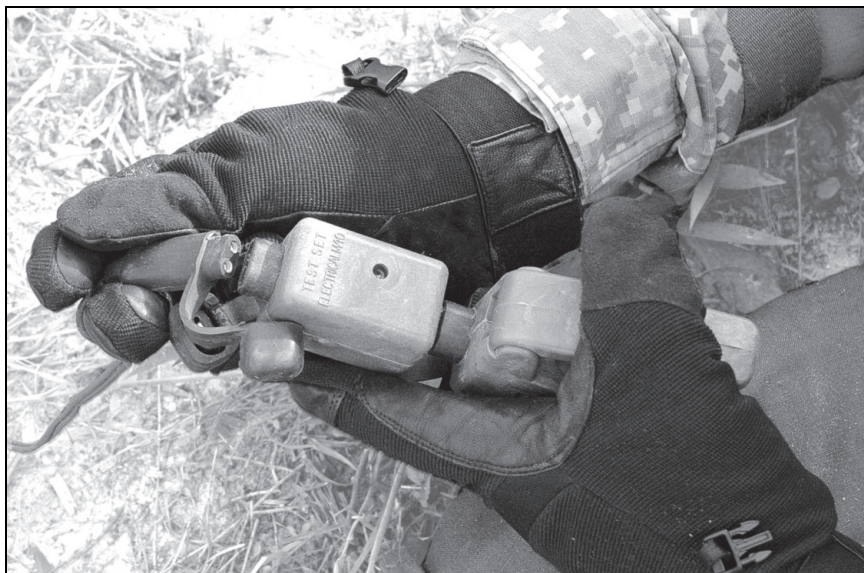
Figure 3-15. Plugging the firing wire connector into the M40 test set
