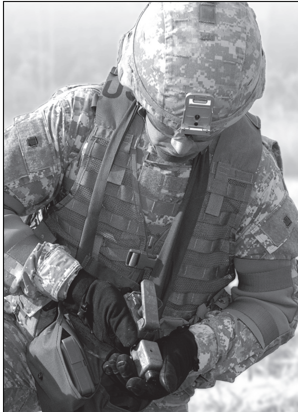
Figure 3-9. Plugging the M40 test set into the M57 firing device
