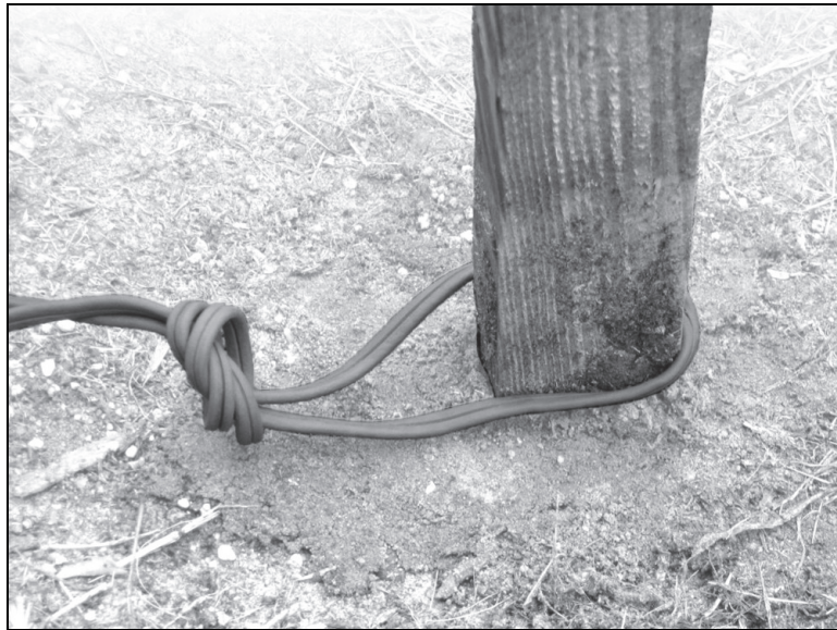
Figure 3-22. Securing the firing wire at the munition emplacement site
