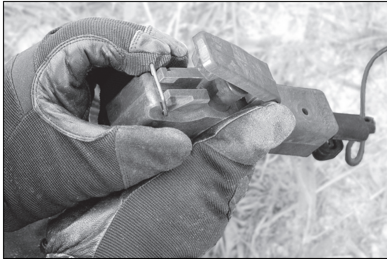
Figure 3-16. Moving the M57 firing device from the SAFE position to the FIRE position
