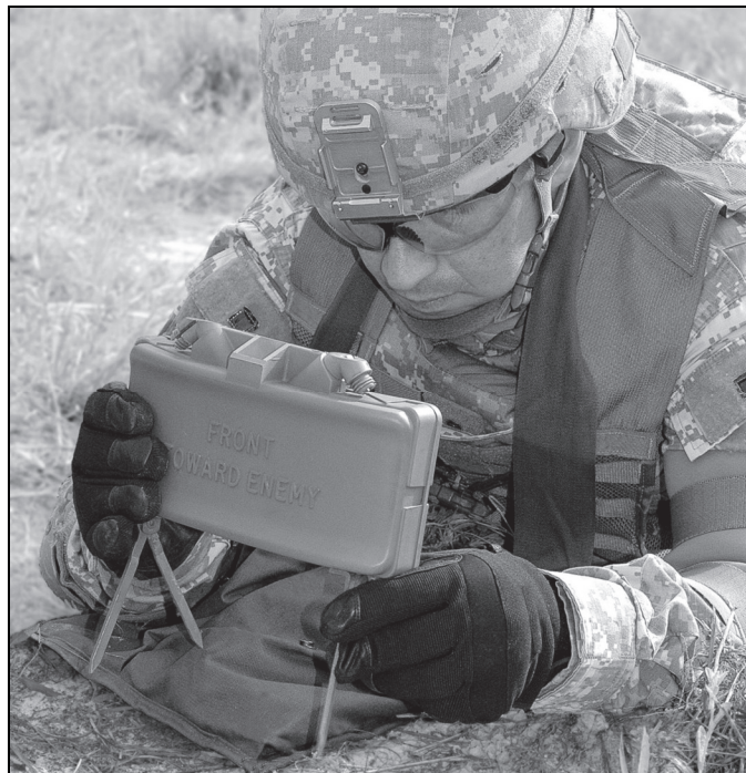
Figure 2-7. Positioning the M18A1 claymore munition with the front facing in the desired area of fire
