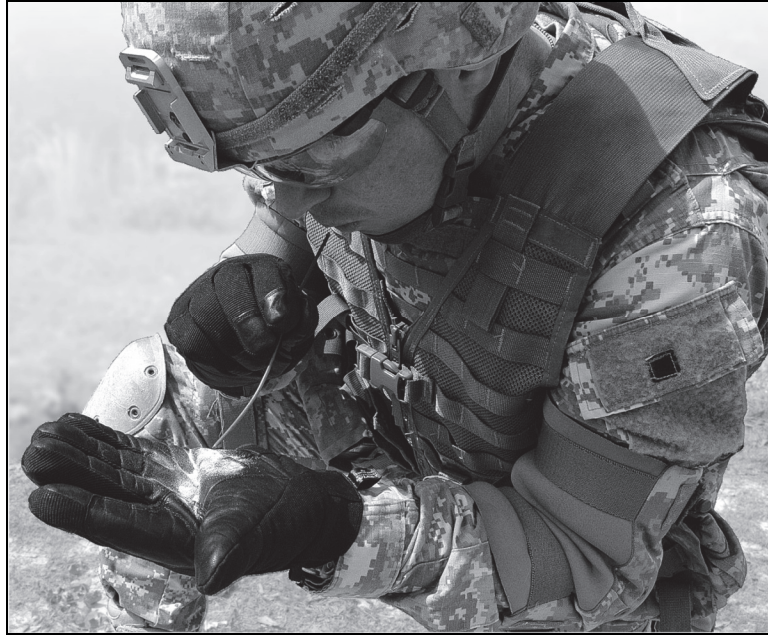
Figure 2-18. Testing for powder in the shock tube
